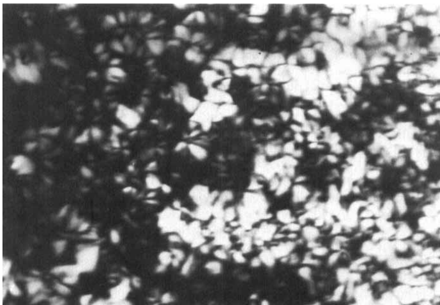
Figure 2. The nematic texture of DACI/70 per cent \text{H}_3\text{PO}_4 system obtained after equilibrating the sample for c. 2 h.
